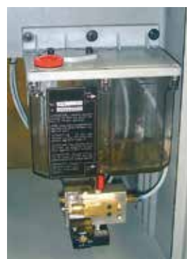
ML Microlubrication system. Available for all series.
